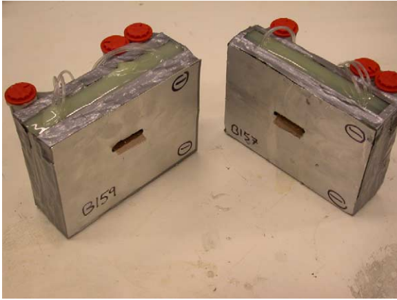
Fig. 8. Ebonex® bipolar lead-acid batteries (6 V).
